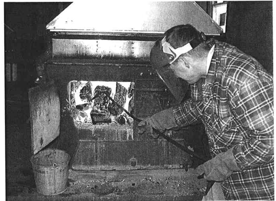
John Geissler, St. John's Arboretum, fires the evaporator in the St. John's Sugar House. Photo by Stephen G. Saupe
